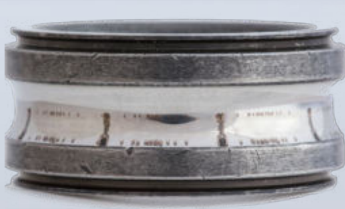
False Brinelling Marks on Bearing Inner Ring
