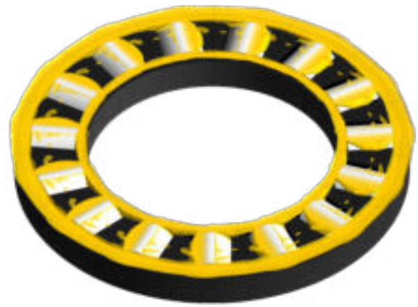
CFD Simulation of the Grease Distribution in an Thrust Roller Bearing
